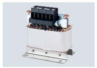
Line reactors smooth the current drawn by the inverter and thus reduce harmonic components in the line current. Through the reduction of the current harmonics, the thermal load on the power components in the rectifier and in the DC link capacitors is reduced as well as the harmonic effects on the supply. The use of a line reactor increases the service life of the inverter.
