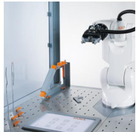
A delicate touch is called for: with great sensitivity, the KR 3 AGILUS fastens micro screws even with a diameter of just 0.8 mm!
