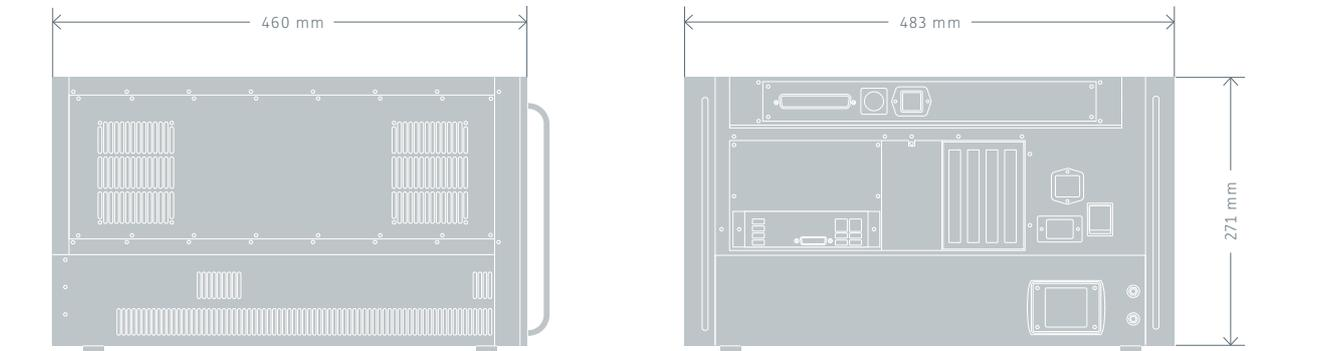
**Space-saving.** The compact dimensions of the housing enable space-saving installation in 19" enclosures or in small protective housings. Despite its compact size, the KR C4 compact offers the entire range of functions of the KR C4 controller.
